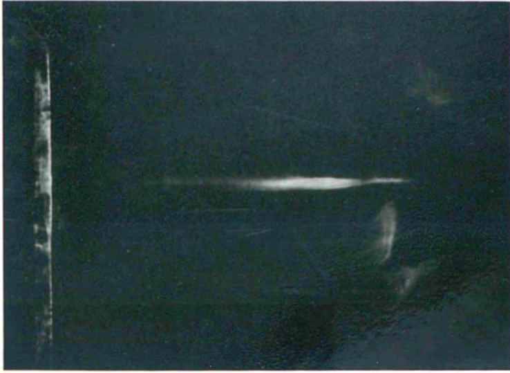
Fig. 5.1.2 Schlieren photographs at t \approx 0 , for various obstacle sizes. Inner electrode diameter 5 cm. Initial conditions V = 30 kV, p_0 = 2.5 torr ( D_2 + 4\% \text{ Ar} )
