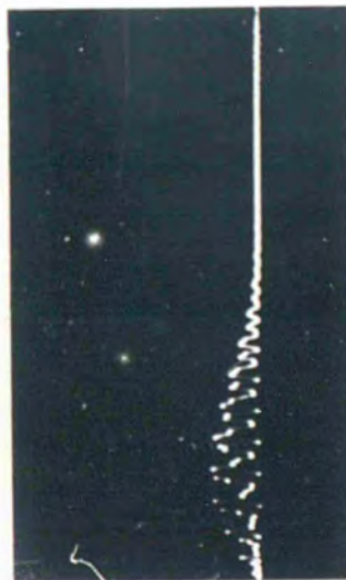
Fig. 4.2.1 Q-switched and mode-locked pulses from a ruby laser
