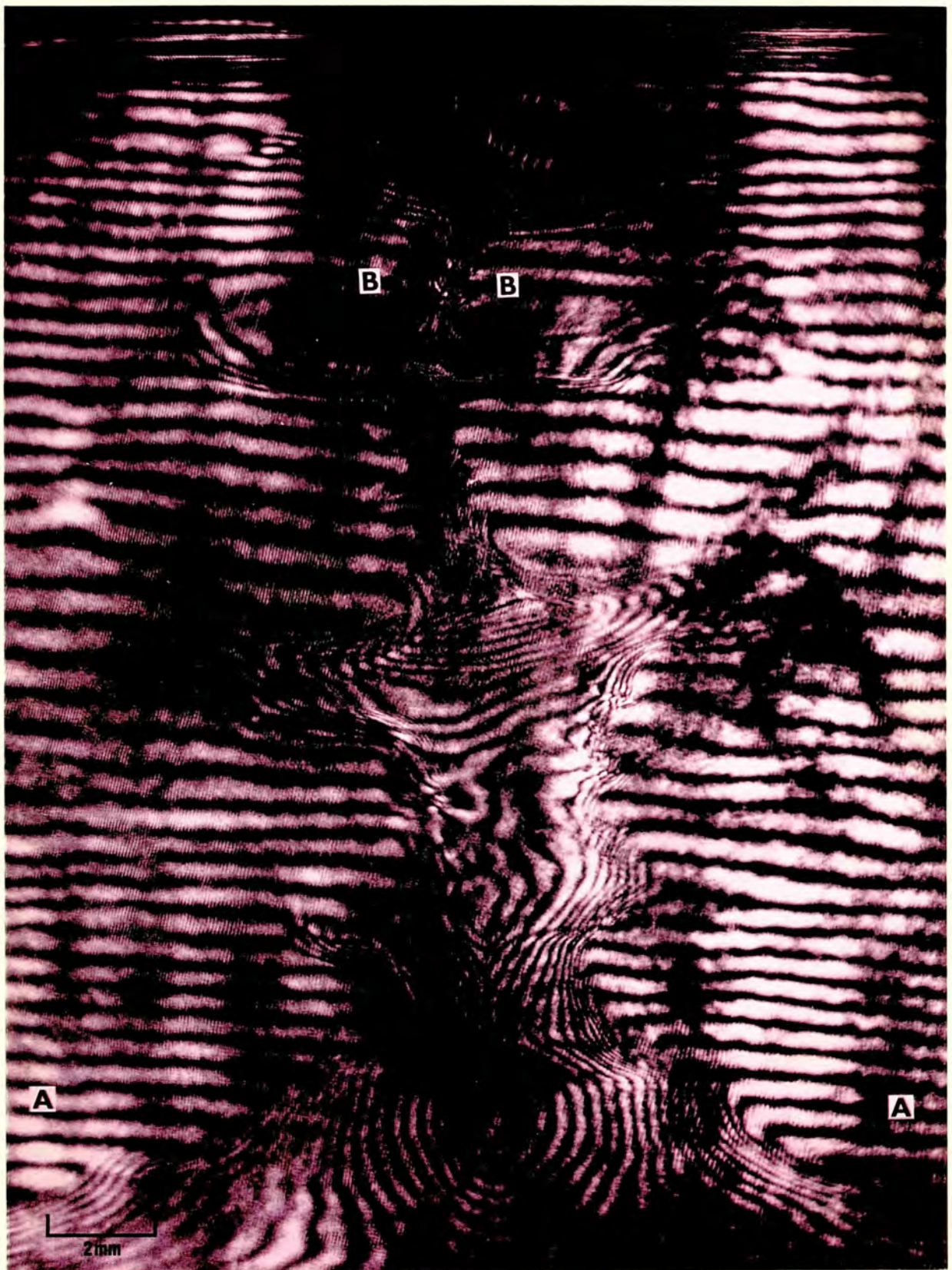
A Mach-Zehnder interferogram of a Plasma Focus discharge near maximum compression ( n_e \sim 5 \times 10^{19} \text{ cm}^{-3} , T_e \sim 2 \text{ keV} , exposure time = 1.2 \times 10^{-9} \text{ s} )
