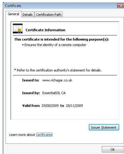
Figure 20 – Certificate details from spoofed web server with SSL
