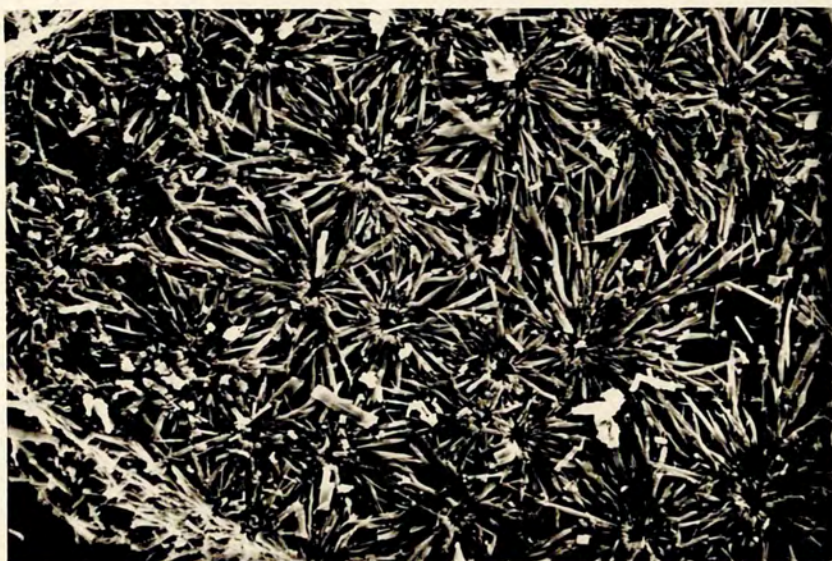
Figure (26): Crystal growth of TTF/DYE complex on platinum mesh electrode as shown by electron microscopy (1mA for 1-0 hour)
