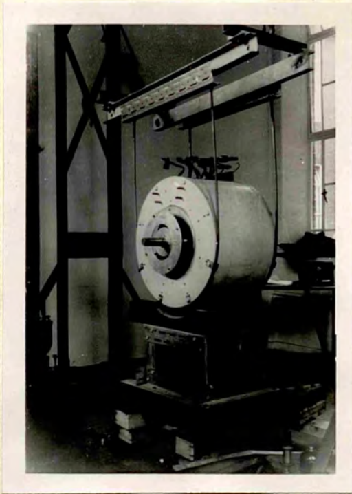
Fig. 22. The small spectrometer being slightly raised for bringing up to the large spectrometer. Two pairs of short studs used for drawing the two spectrometers together can be seen on the upper part of the iron plate.
