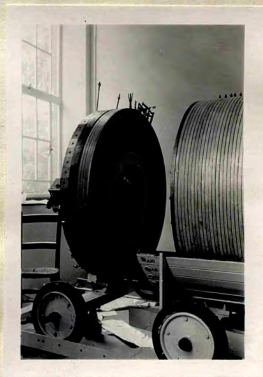
Fig. 12. The left hand end plate showing the pole piece. The crystal is withdrawn into the hole at the centre for protection. The corner blocks with the holes are on the left.
