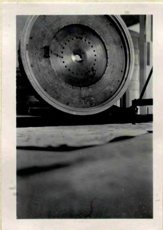
Fig. 11. The right hand end plate. Note the bevelled hole and bush at the centre of the iron plate, the pumping holes and bracket for the rotating coil.
