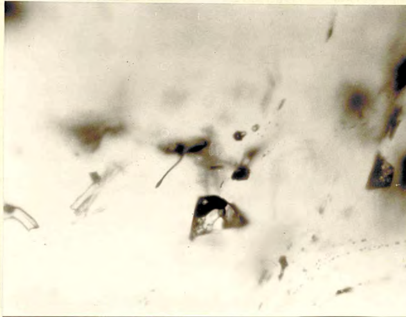
Plate 30. Photomicrograph of fluid inclusion within sample GL.26, containing solid phases as daughter minerals. Horizontal edges of the photograph \sim 300 \mu\text{m} .
