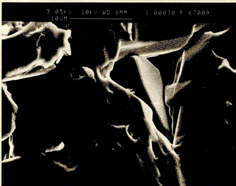
Plate 31. SEM view of opened inclusion within sample GL.30, showing a Cu-Fe sulphide crystal. (Probably chalcopyrite).
