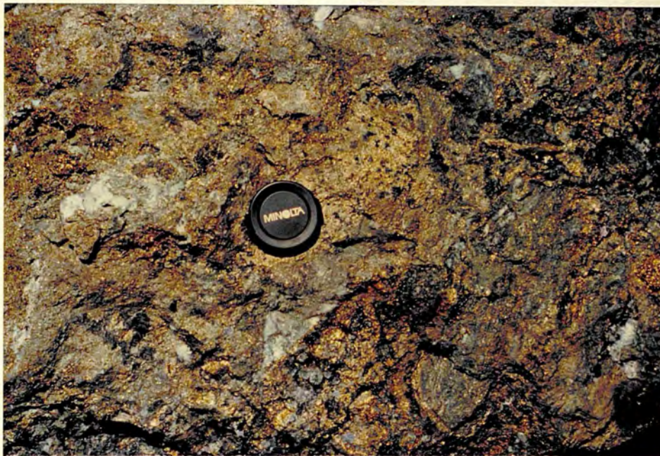
Plate 14. The feature of the brecciated ore, showing a massive ore composed of galena (dark grey) and chalcopyrite and pyrite (yellow). Locality: tunnel T.400.
