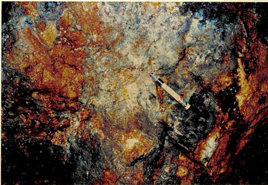
Plate 13. The features of parts of ore zone in tunnel T.580, mainly composed of chalcopyrite (which is partly altered to malachite and azurite) associated with quartz filling the breccia; showing an advanced argillic alteration of the host rock.
