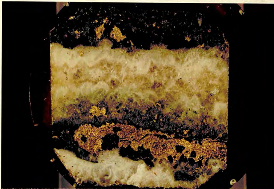
Plate 22. The feature of stratified ore, showing banded sphalerite (light brown) at the top and chalcopryite (yellow) containing pyrite aggregate (dark brown/black); associated with quartz vein. Diameter of the mounting is 3 cm.
