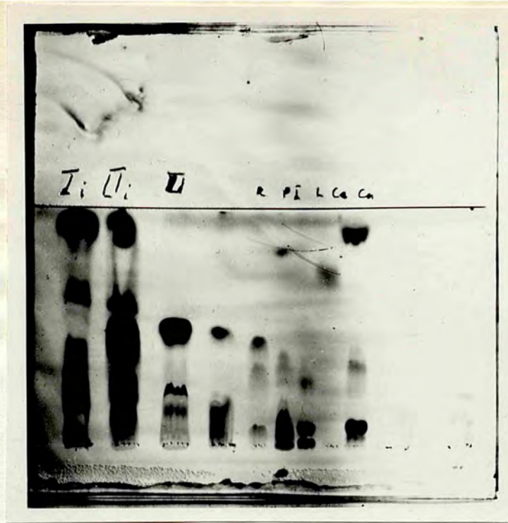
Fig. 6. Thin layer chromatogram of regions I (Fractions 3 and 4), II (Fractions 13 and 14) and III (Fractions 23-30) of the silicic acid column of the butanol extract. The plate was chromatographed in C:M:H 2 O, 80:30:3 and developed in a saturated iodine tank.
