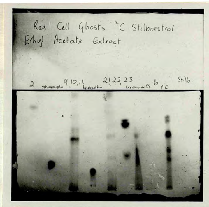
Fig.29a. Thin layer chromatogram of Fraction 2, Fractions 9-11 and Fractions 21-23 of the silicic acid column of the ethyl acetate extract of the stilboestrol inhibited ghosts. The plates were chromatographed in C:M:H 2 O, 80:30:3 and developed in a saturated iodine tank.
