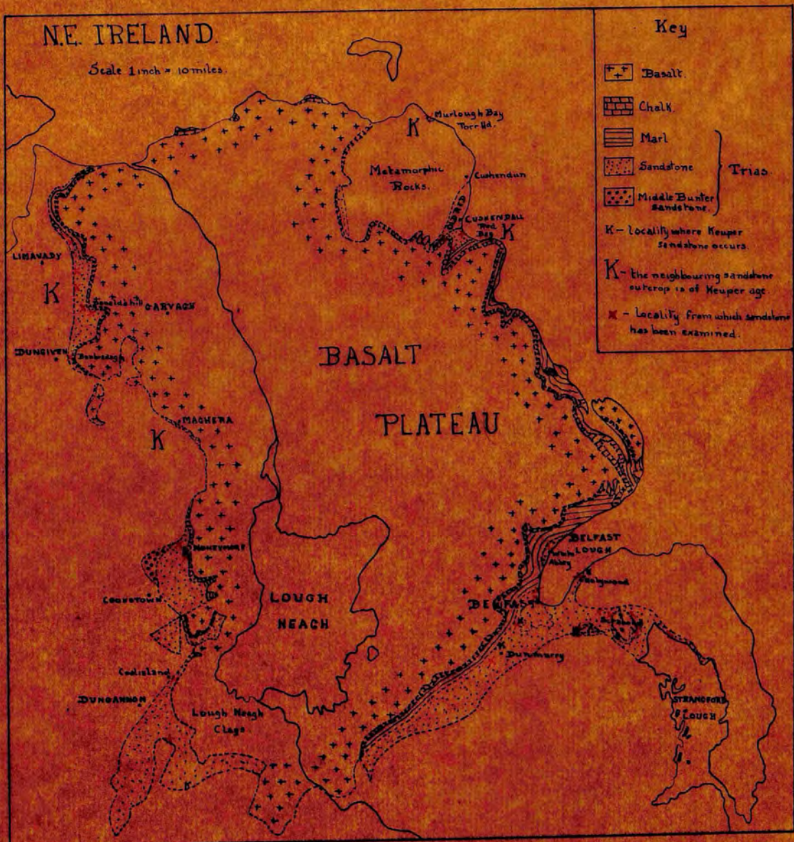
MAP SHOWING THE DISTRIBUTION OF BUNTER & KEUPER SANDSTONE AS DETERMINED BY THE GEOL. SURVEY & LOCALITIES FROM WHICH SANDSTONE HAS BEEN EXAMINED DURING THE PRESENT INVESTIGATION.
