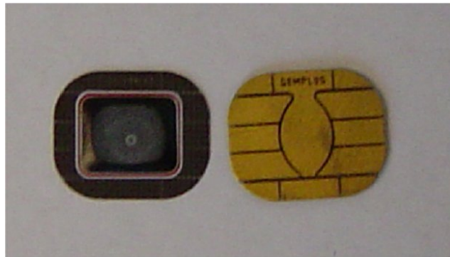
Figure 3.2: A front and rear view of a micromodule before it is set into a plastic card.
