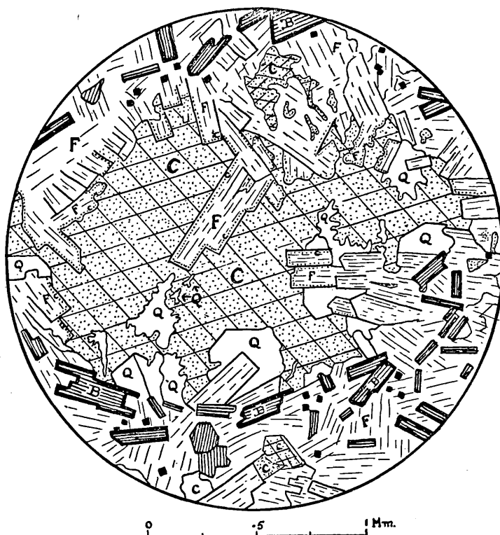
FIG. 4.—Drusy cavity in a kersantite (No. 233) showing the replacement of quartz and felspar by calcite. C = calcite; F = felspar; Q = quartz; B = biotite. Dots within the margin of the felspar represent speckling with calcite.
