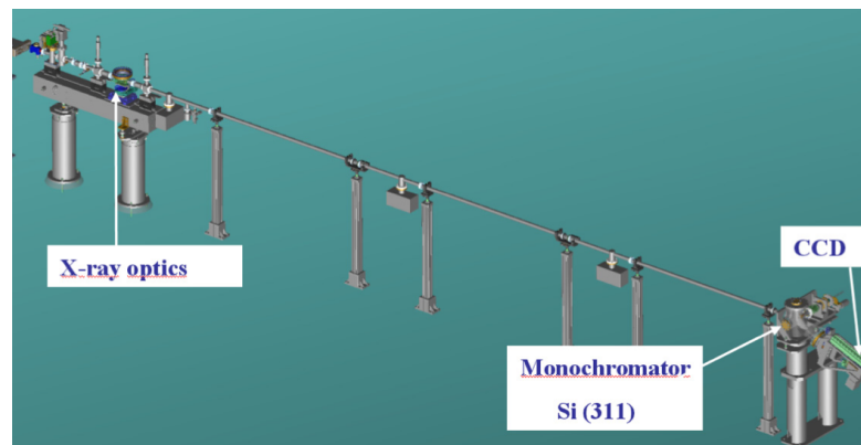
Figure 4.2: Overview of the diagnostics beam-line starting from the entrance absorber [27].
