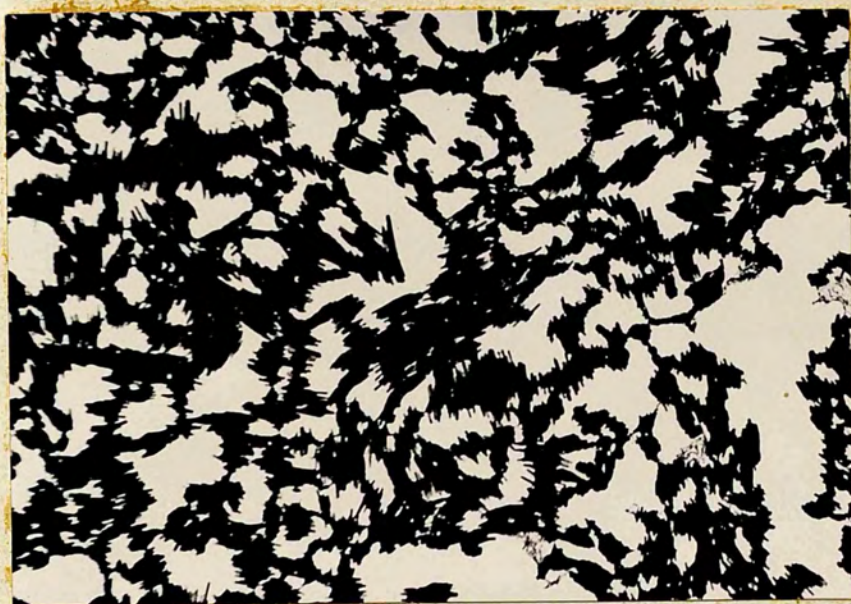
Figure 21. Selenium on (111) Na Cl x 8000. 500 Å thickness.
