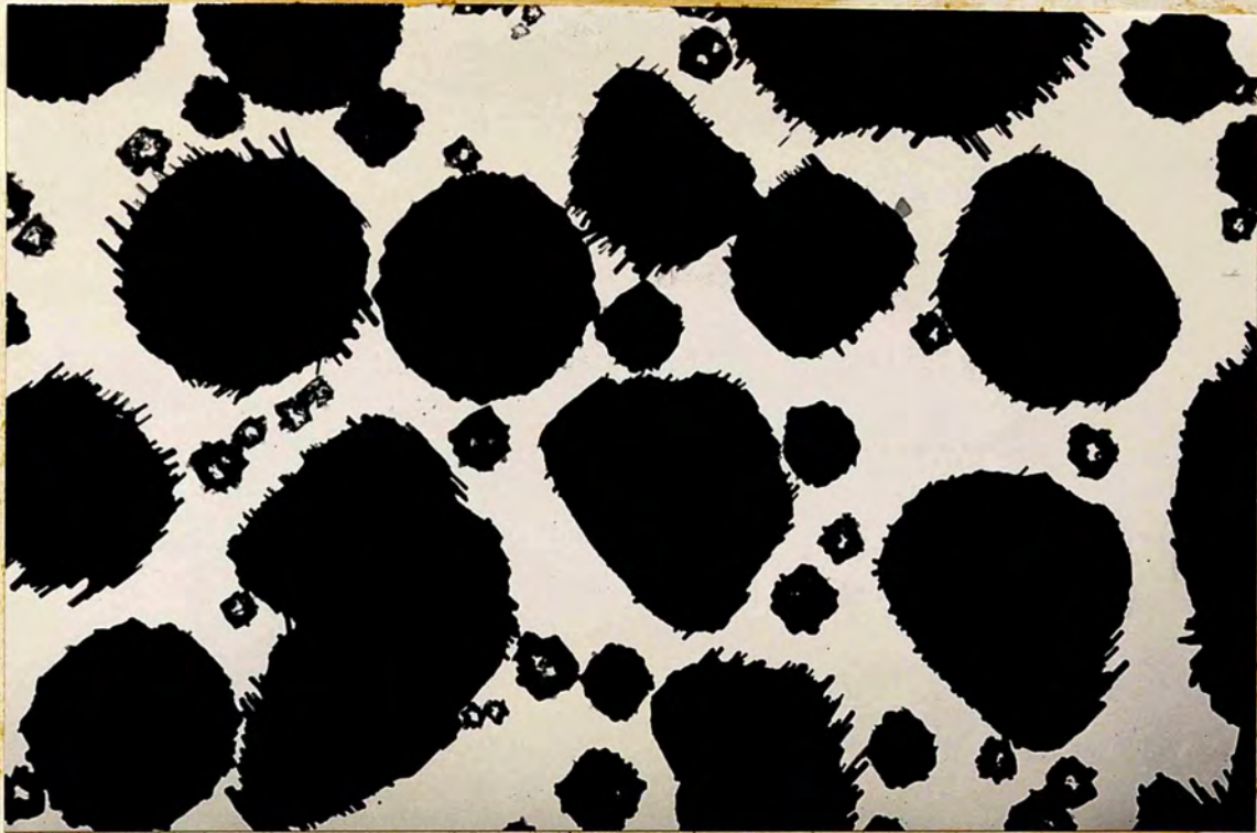
Figure 24. Selenium on (100) K Br. x 8000.
