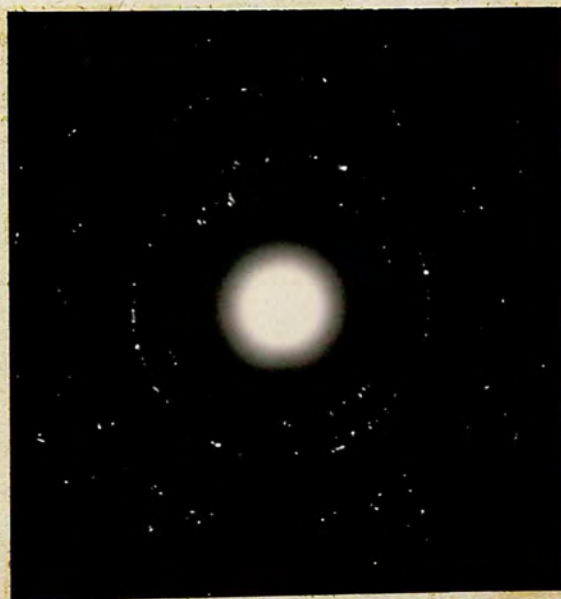
Figure 22. Diffraction pattern from selenium on (111) Na Cl.
