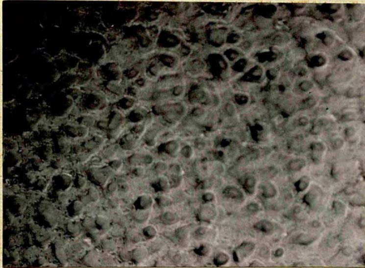
Figure 10. (100) potassium bromide surface annealed at 420^{\circ}\text{C} .
