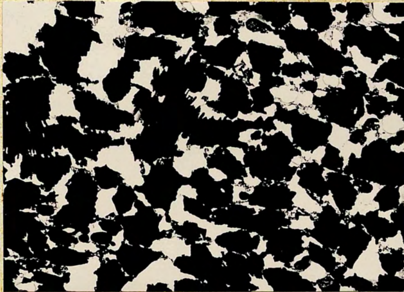
Figure 19. Selenium on (110) Na Cl x 8000 700 Å thickness.
