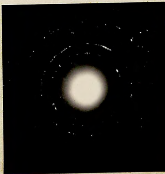
Figure 20. Diffraction pattern from selenium on (110) Na Cl.
