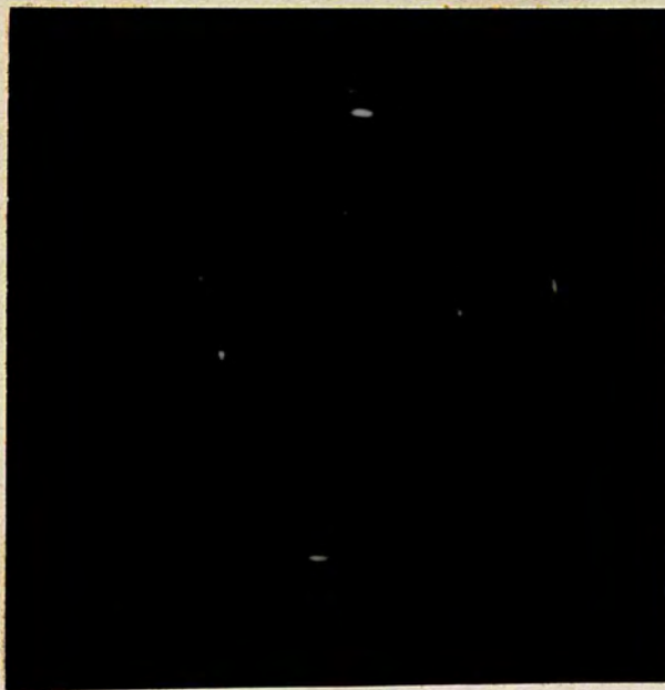
Figure 42. Diffraction pattern from selenium film with superimposed grid bars.
