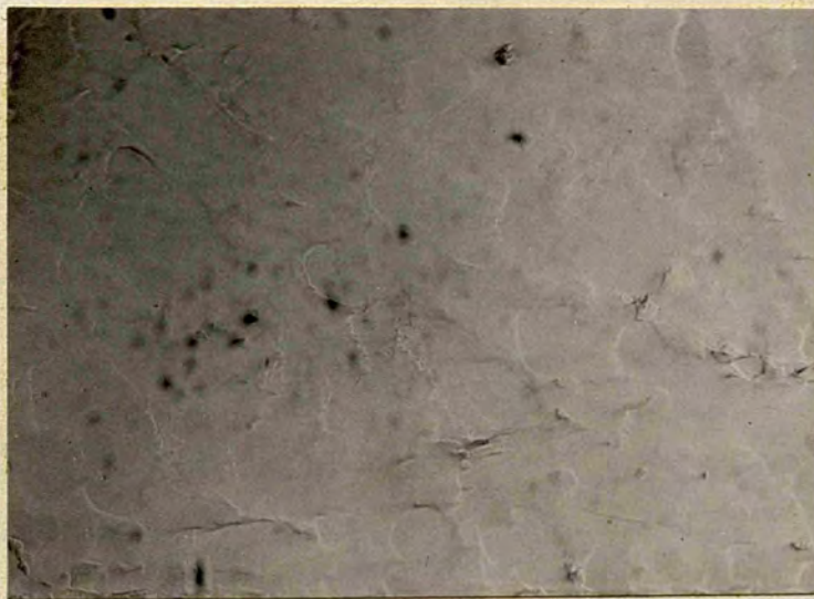
Figure 11. (100) potassium bromide surface annealed at 370^{\circ}\text{C} .
