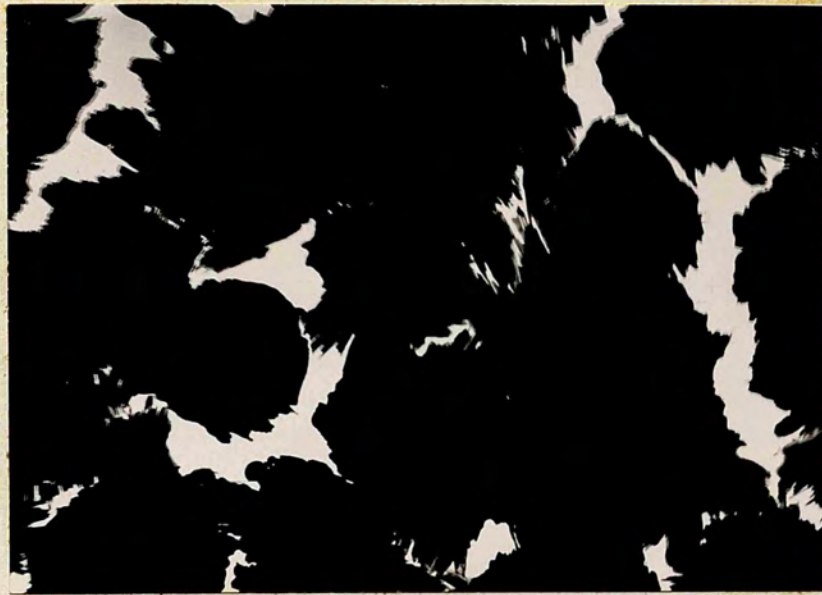
Figure 17. Selenium on (100) Na Cl x 8000. 2000 Å thickness.
