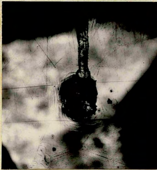
Figure 16. Pit left by thermocouple in substrate surface. x 50.
