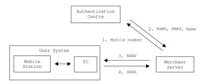
Figure 1: GSM-e-commerce identity authentication process.
