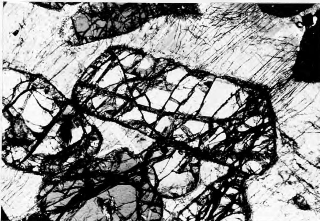
PLATE 4.14. Tabular morphology with well- developed pinacoid faces.
