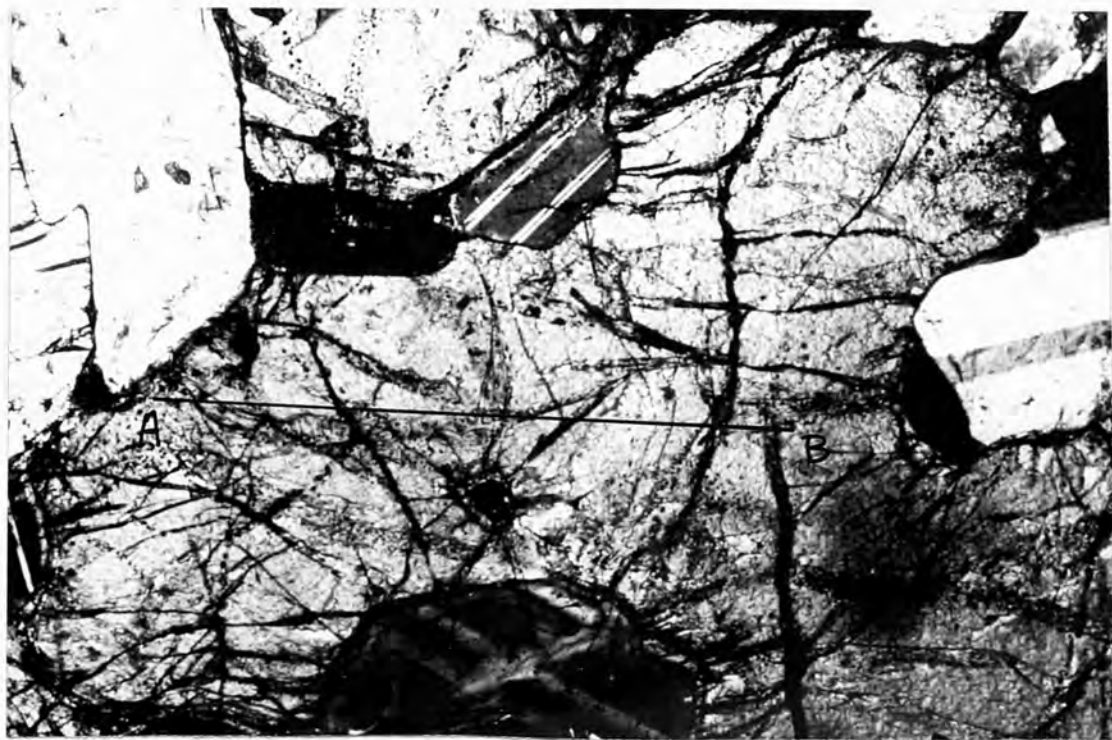
PLATE 4.7. Irregular, amoeba-like morphology showing trajectory of microprobe scan (A - B).
