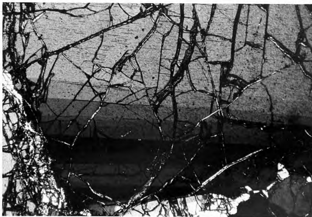
PLATE 4.15 Development of strain lamellae in the olivine crescumulate.
