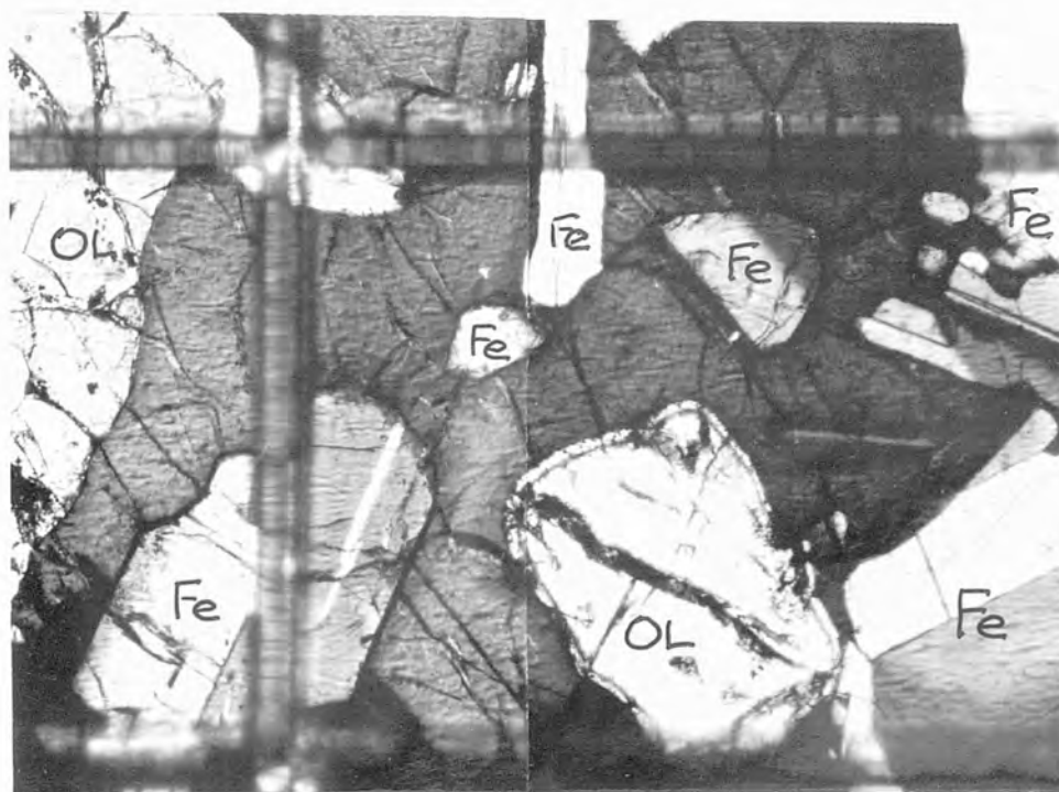
PLATE 4.20 (a). Poikilitic clinopyroxene enclosing olivine (OL) and tabular feldspar (Fe). 0.1mm
