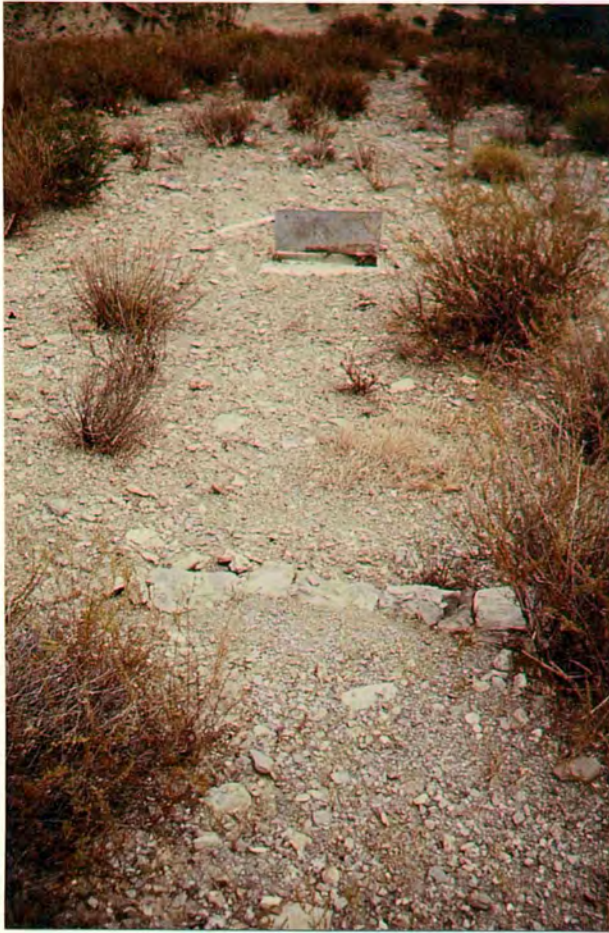
Photograph 5.1 Runoff plot and Gerlach trough on the conglomerate S1T9
