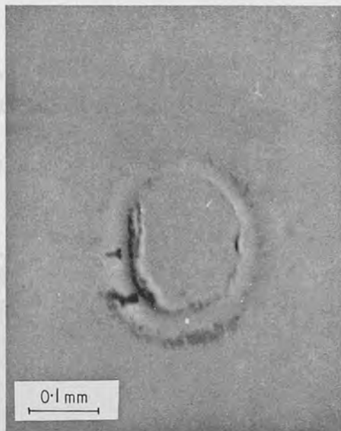
Figure 3. Direct photograph of the damage caused to a glass surface bearing a 1000 \text{ \AA} gold film by using a lens of 25 cm focal length to focus a 2 W laser beam onto the surface for a period of 1 s.
