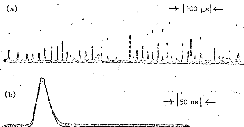
Fig. 3.2 (a) Intensity output of a 'free-running' ruby laser (b) The 10 \text{ MW/cm}^2 output of a 'Q' switched ruby laser
