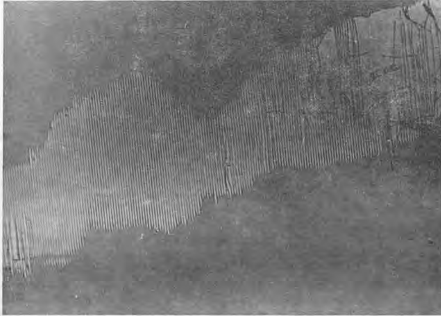
Fig.17. Grating of the type produced using a 'low energy' ruby laser pulse (200 Å gold film illuminated by a 0.06 J/cm 2 ruby laser pulse).
