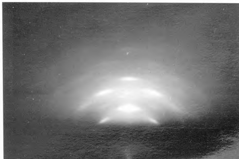
PLATE (6.7) High energy reflection electron diffraction pattern of an U.H.V. grown dysprosium film.
