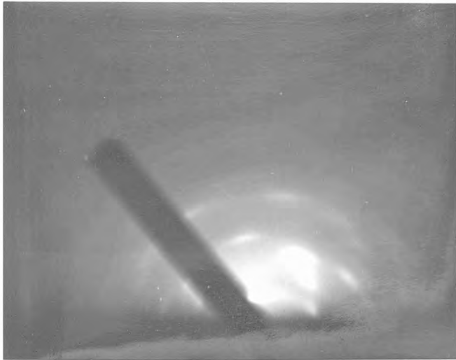
PLATE (6.3) High energy reflection electron diffraction pattern of a U.H.V. grown terbium film before thermal modulation.
