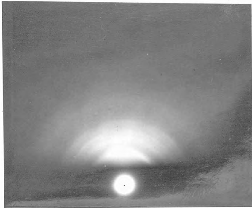
PLATE (6.5) High energy reflection electron diffraction pattern of an O.H.V. grown terbium film before thermal modulation.
