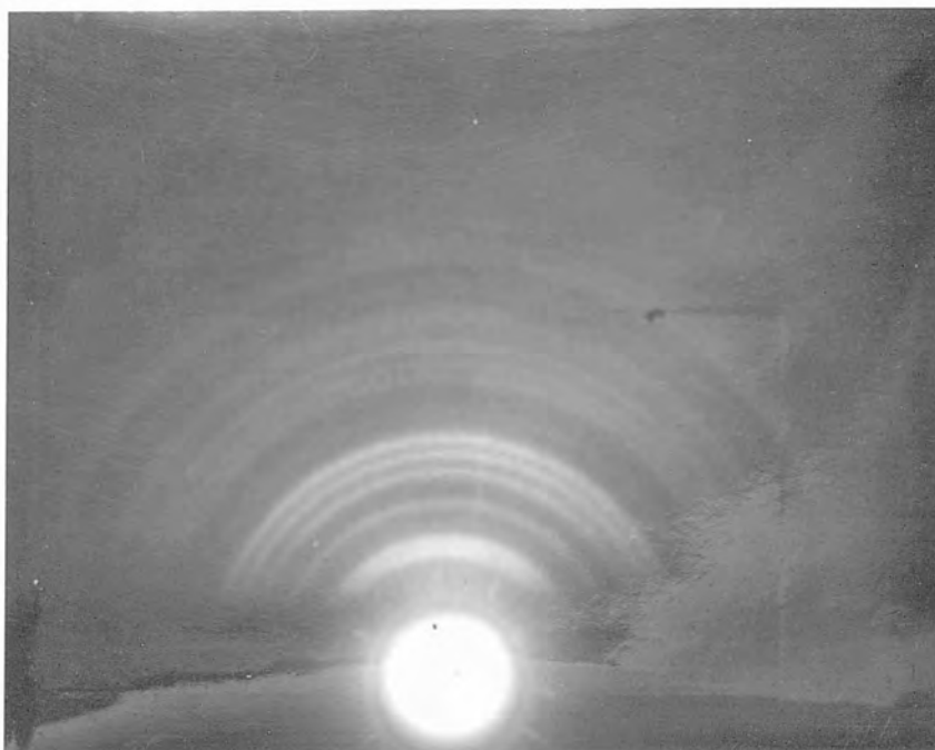
PLATE (4.5) High energy reflection electron diffraction pattern of a 1200 Å cadmium sulphide film. Substrate temperature 185°C.
