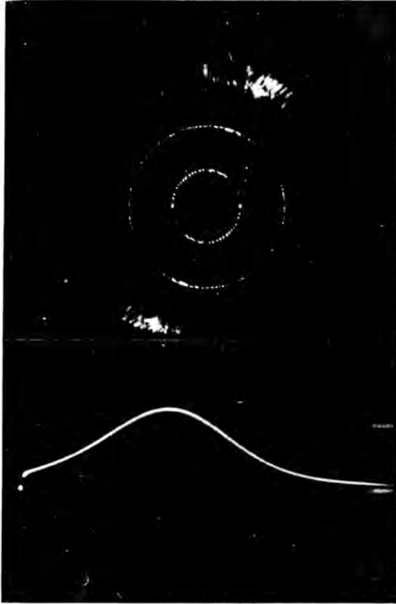
Fig. 2(b). Output spectrum of a Pockels cell switched giant pulse ruby laser. Time scale: 100 nsec/cm. Peak power 100 kW.
