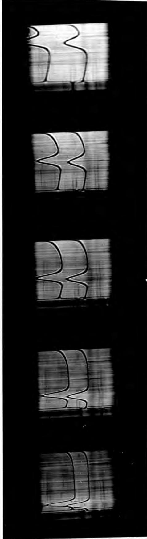
Plate 3.1 Ultracentrifugation of glucoamylase I (upper trace) and glucoamylase II (lower trace) at 59780 rpm. Schlieren photographs taken after 29, 52, 78, 104 and 134 minutes from start.
