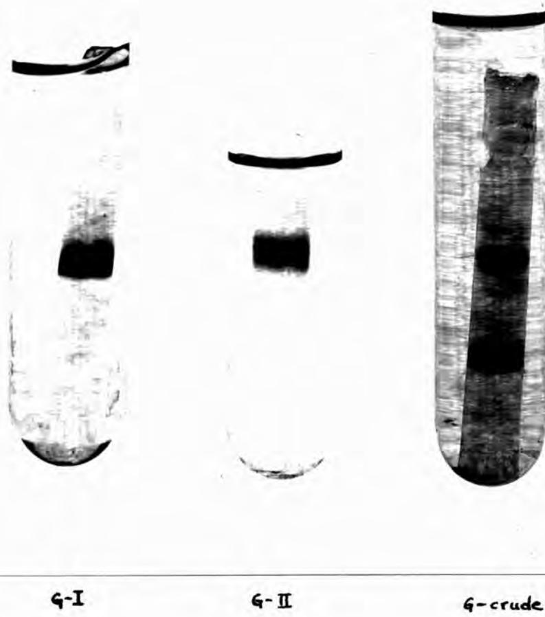
Plate 3.2 Electrophoresis of glucoamylase I (G-I), glucoamylase II (G-II) and crude glucoamylase (G-crude) in 7.5% polyacrylamide gel at pH 8.9 (TRIS/HCl) and 5mA per tube.
