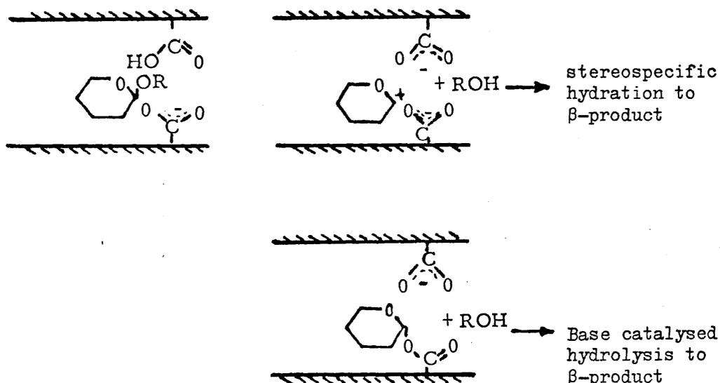
**SCHEME 6.2** Proposed mechanism<sup>100</sup> for enzyme hydrolysis proceeding with retention of anomeric configuration of product.
