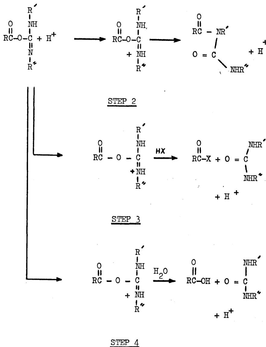
SCHEME 6.1 Proposed mechanism<sup>75</sup> for carboxyl group modification by a water soluble carbodiimide.
