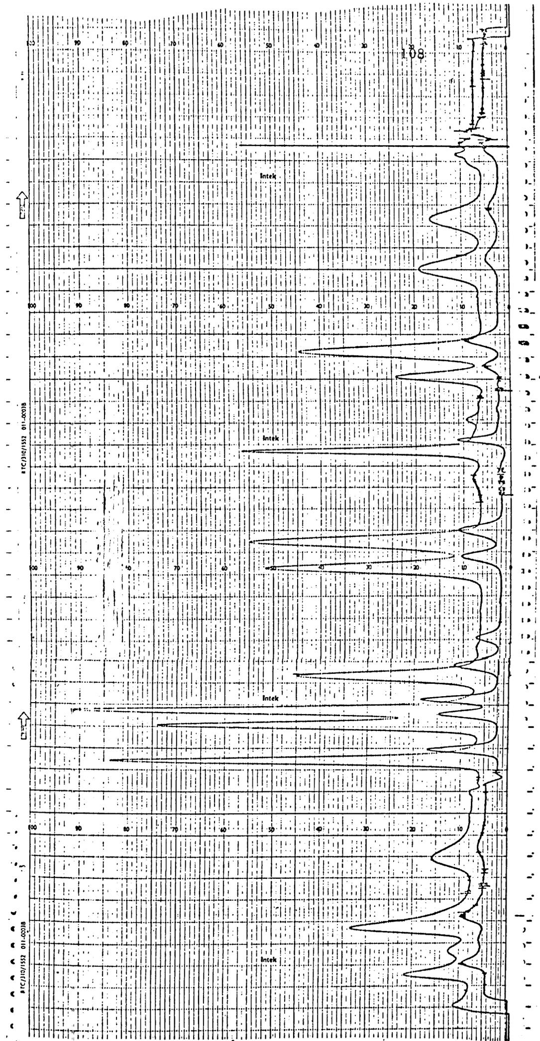
**FIGURE 4.3.** Amino-acid analysis of glucoamylase II after 72 hour acid hydrolysis.
