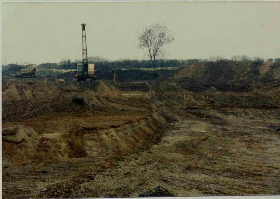
Plate 31. Stoke Goldington - section at point F (October, 1983). Showing extraction of the fluvio-glacial gravel (l) to the surface of the terrace gravel (j).
