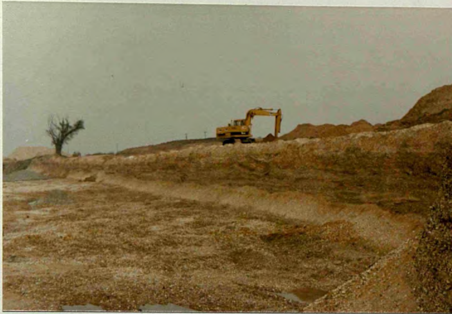
Plate 1. Site 2. Broughton - showing horizontally bedded gravel (2.5-4m) extracted to the local bedrock (Oxford Clay).
