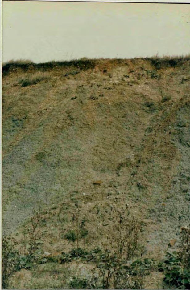
Plate 5. Site 19. Ridgmont - showing thin layer of fine gravel (0.5-1m) overlying chalky till.
