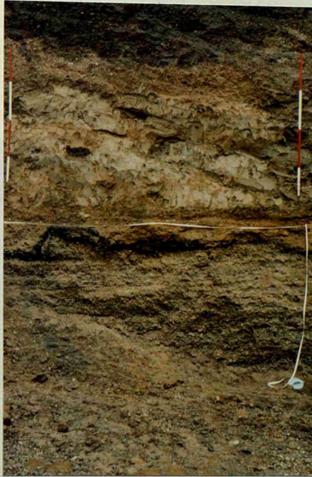
Plate 30. Stoke Goldington - section at point F (October, 1983). Showing terrace gravel (j) overlain by clay (k), and with fluvio-glacial gravel (l) on top.
