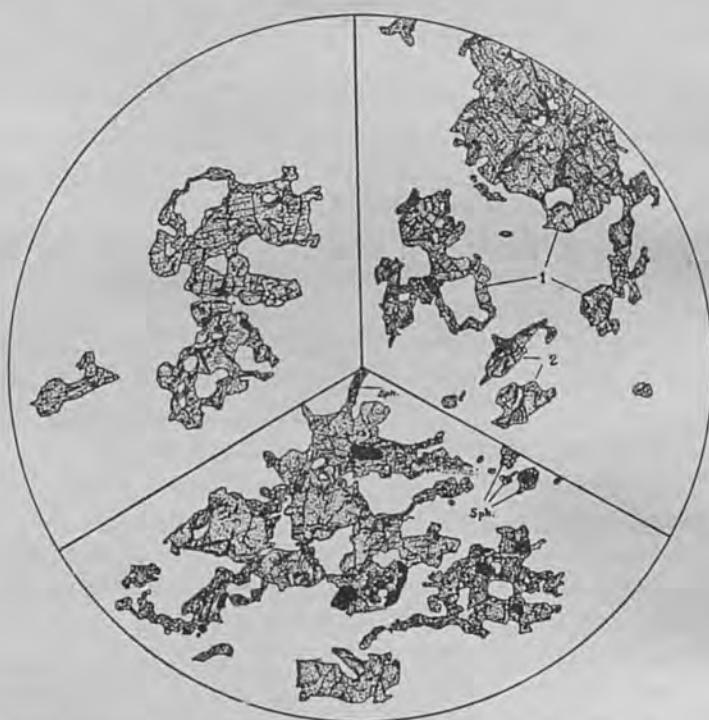
FIG. 4.—Poikiloblastic crystals of aegirine-augite in siliceous granulite (slice 200, from Allt Torr an Tairbh). The pyroxene areas in each sector of the diagram are optically continuous (except where the contrary is indicated), even where no direct connexion occurs. The background consists of a granular mosaic of quartz, together with some potash felspar.
