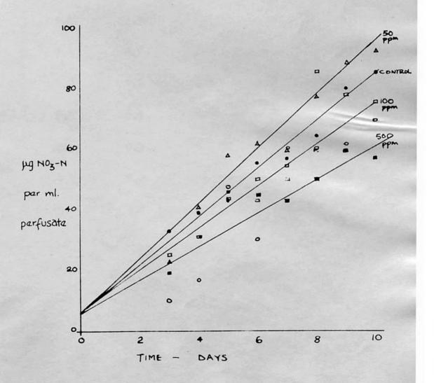
The nitrification rates when enriched soil was perfused with ammonium sulphate solution in the presence of the herbicides listed and at the concentrations indicated.
