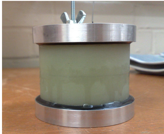
Figure 7.16: Photograph showing the fibreglass and aluminium cell used for testing the strength of the stycast seals.
