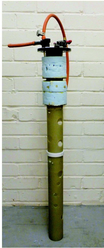
Figure 7.19: Photograph of the fibreglass insert attached to the aluminium top-plate. The receiver coil wiring and SQUID sensor are not yet included.
