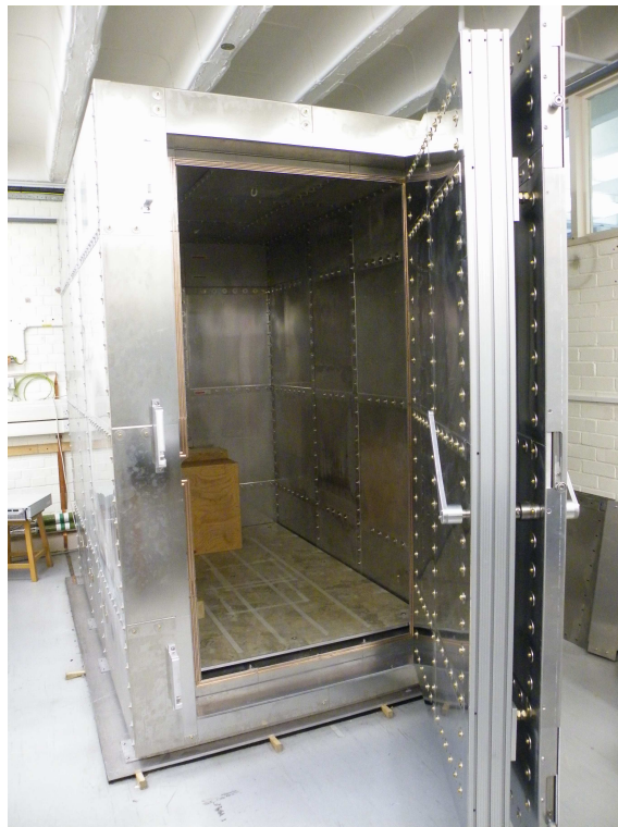
Figure 7.1: Photograph showing the rebuilt magnetically shielded enclosure.
